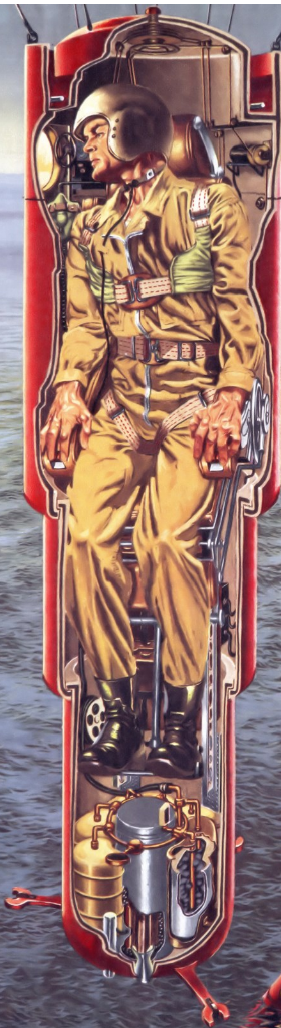
Emergency capsule is ejected from rocket ship with crewman inside, drops into sea. Speed is slowed by metal chute, impact is cushioned by small rocket in capsule base. The picture shows radar-equipped plane, rescue vessels converging on area to pick up four crew members—one in sea, two being slowed by rockets, and one (foreground) still so high rocket hasn't blasted yet. Cutaway shows man in capsule, strapped to contour chair, with rocket and frozen air under feet. Metal arms on base guide capsule during ejection
